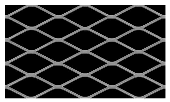
LW Pitch:50.80mmStrand Width:3.05mmSW Pitch:22.58mmThickness:1.50mmWeight:3.20 kg / m2Open Area:73%
